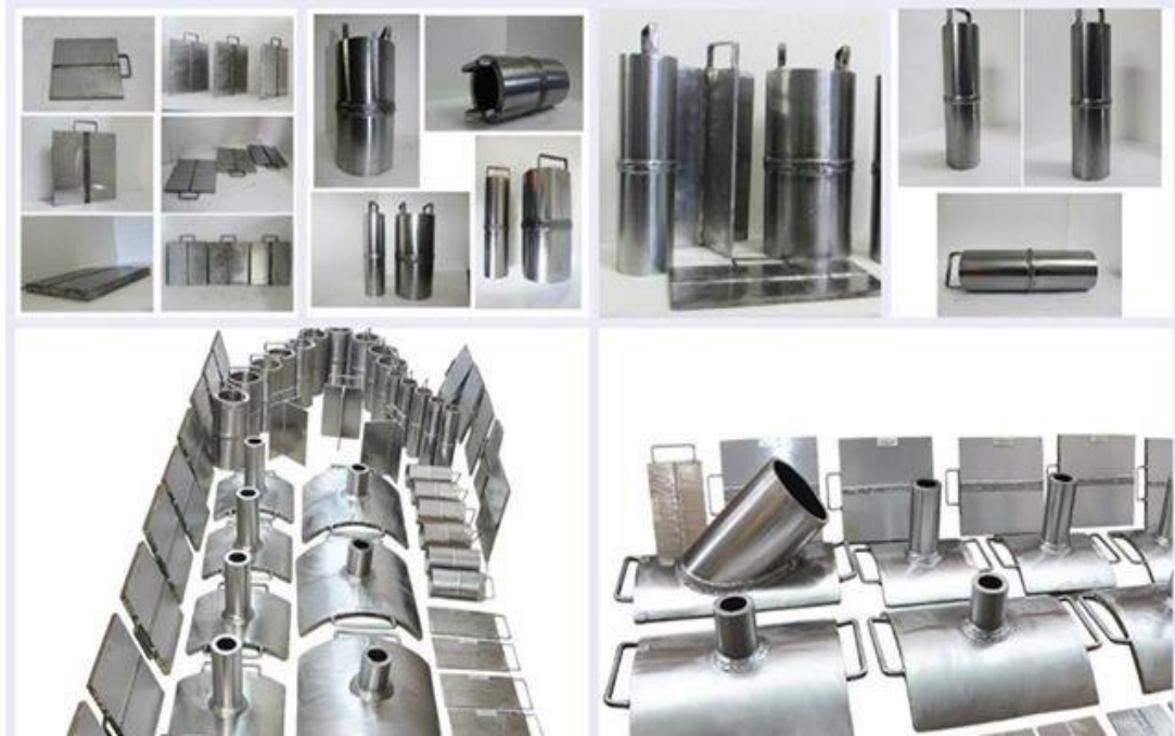
Flawed Specimen Test Components
